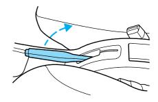
1. Set the parking brake and ensure the gearshift is securely latched in P (Park).
